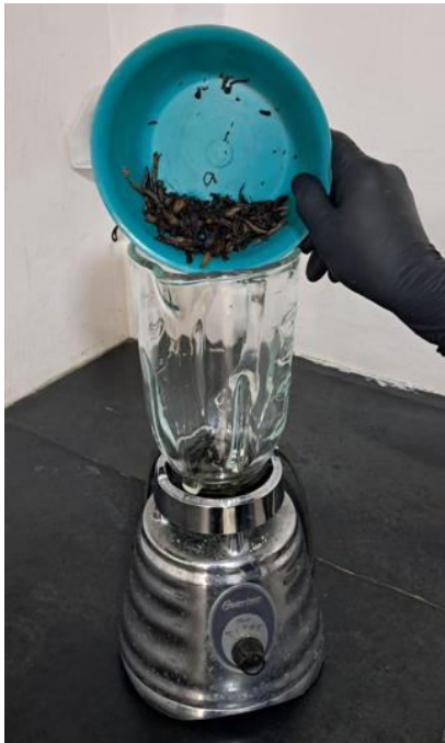
Figure.11 Blend the roots in 150 ml of water for 10 seconds at low speed followed by 10 seconds at high speed.
