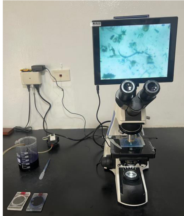
Figure.17 Identify and enumerate the nematodes present in the aliquot using an Olympus BH microscope at 4x magnification.
