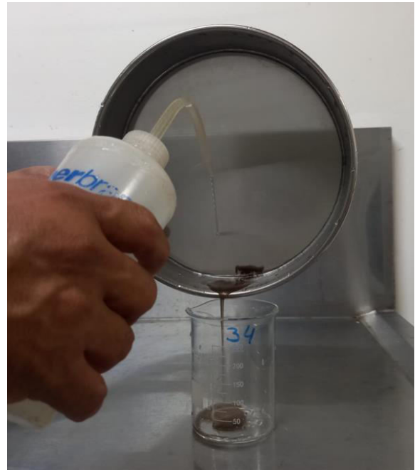
Figure.14 Collect and wash the nematodes of the 0.025 mm sieve into a 250 ml beaker.
