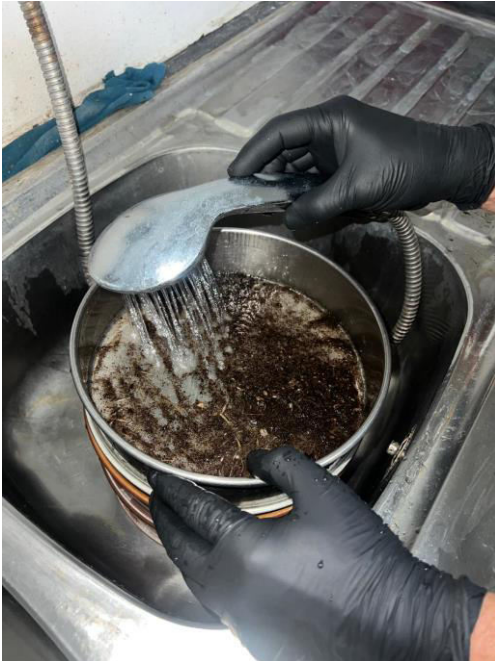
Figure.13 Wash the 0.25 mm sieve for 2 minutes and then the 0.106 mm sieve for 1 minute.
